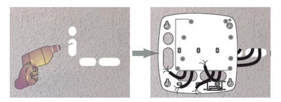
b. Screw the back of the panel to the wall, using either drywall screws or threaded wall anchors.
